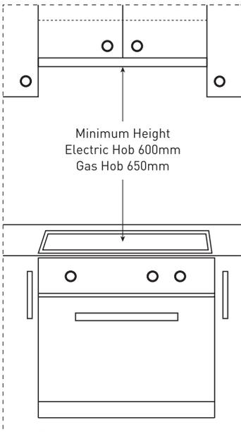
The image to the left, illustrates the minimum height from the hob surface to the underside of the rangehood.
