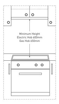
The image to the left, illustrates the minimum height from the hob surface to the underside of the rangehood.
